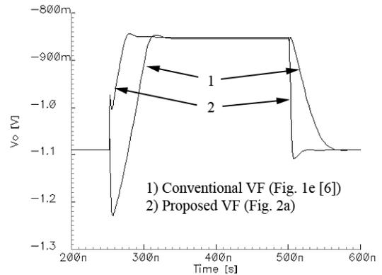
Figure 4. Transient response of the conventional and proposed voltage followers in Fig. 1e and 2a respectively, for an input signal of  $300\text{mV}_{pp}$  at  $2\text{MHz}$  with a load resistor of  $1\text{k}\Omega$ .
