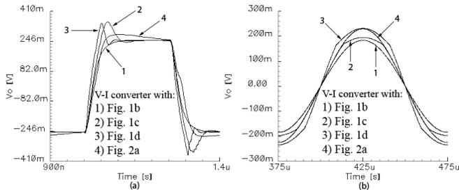
Figure 6. Transient response of the V-I converter using the voltage followers in Fig. 1 for a) a square input signal of  $0.5V_{pp}$  at 2MHz and a capacitive load of  $C_L=15pF$  and b) a sine wave of  $0.5V_{pp}$  at 10kHz and a resistive load of  $1k\Omega$ .
