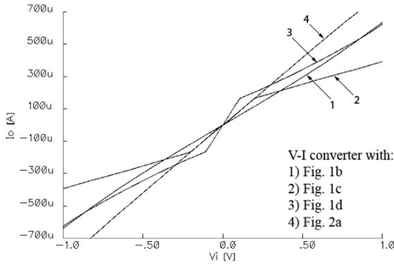
Figure 5. Dc transfer characteristic of the V-I converter using the voltage followers in Fig. 1.
