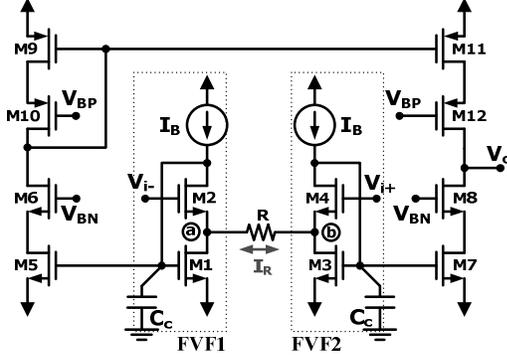
Figure 3. Highly linear V-I converter with conventional FVF used to test the performance of circuits in Fig. 1b-1d and proposed structure in Fig. 2a.
