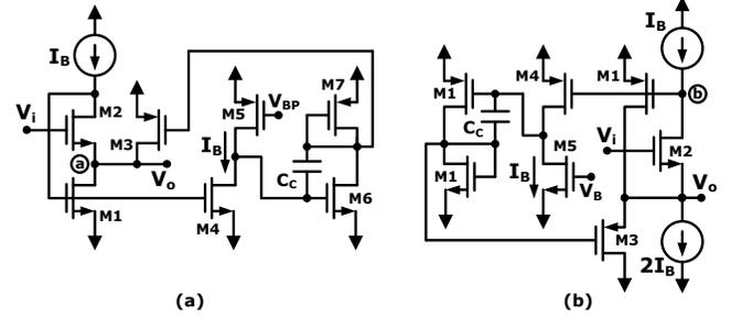
Figure 2. Proposed class AB voltage followers based on the modification of the FVF in a) Padilla-Cantoya [6], and b) its extended output-swing version.
