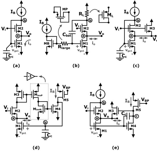
Figure 1. Voltage followers: a) conventional class A FVF in [1], b) Class AB version by Ramirez-Angulo [3], c) Class AB version by Jimenez [4], d) Class AB version by Centurelli [5], and e) Class AB version by Padilla-Cantoya [6].
